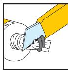
2. Cut the end off the protective film
